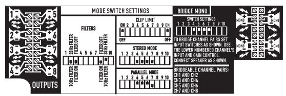
Speaker connection diagrams and "MODE" switch settings are printed on a rear panel label, as shown, above.
